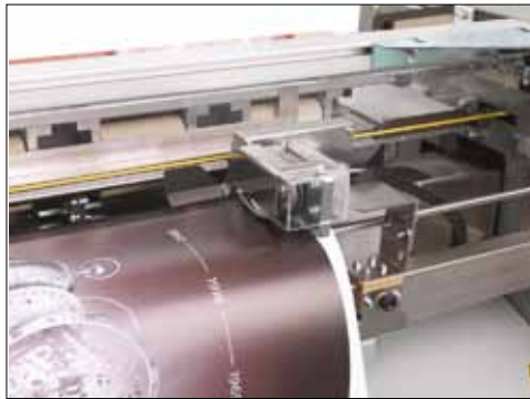
The sensor automatically follows the prints
