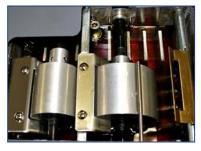
Using a specially formulated EVA glue creates a stronger bind and allows the binding of a wider range of paper types and weights. Binding with this new type of glue and with the addition of the second glue applicator drum, the DB-280 ensures a stronger bind and a quality finish.
